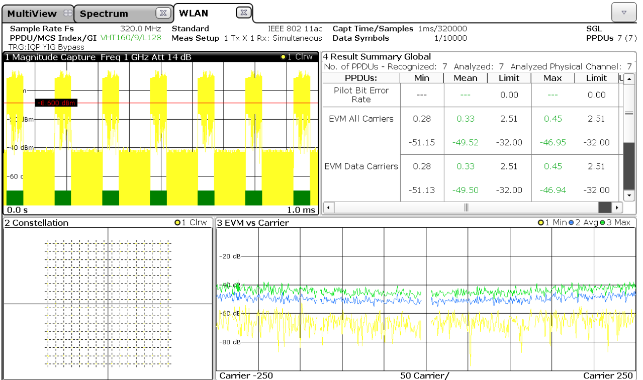
Measured EVM for an IEEE 802.11ac signal with 160 MHz bandwidth
